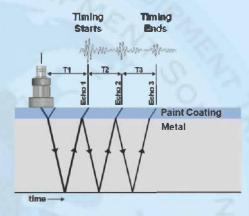
With multiple echo, readings are taken by measuring the time delay between any three consecutive backwall echos. The time of T1 (coating thickness) is ignored. The times of T2 and T3 are equal to the time that it takes to travel through the metal. Only by looking at three echoes can the measurements be automatically (whereT2=T3).
