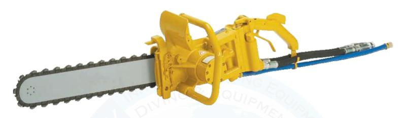
The **DS11** Diamond Chain Saw is specifically designed to cut solid concrete underwater. Cuts square corners without over-cut and can plunge cut sea walls up to 18" thick. Two available bar lengths (15" and 18") and two different chains depending on the amount of rebar and hardness of the concrete.
