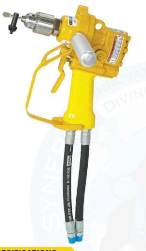
The Stanley **DL07** hydraulic drill is a forward/reverse, variable speed drill with a 1/2" keyed chuck for underwater drilling applications. The DL07 has more than enough torque to drill most steel, masonry, wood or coral. A two position assist handle and trigger guard are standard. See chart below for speeds at select gpm of hydraulic flow. Painted hi-visibility yellow.
